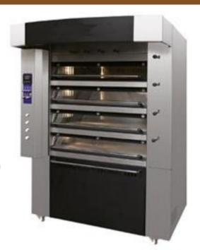
The Mini Vapor Tube Oven is a static oven which means there are no fans to dry out your baked goods. The most important characteristics of this oven is the unique heat heating system. Heat is supplied by a dense network of closed vapor tubes in which hot steam circulates. The baking chambers on each deck are wrapped by these vapor tubes in and around the entire deck, each steam tube is individually tested certified at our factory
