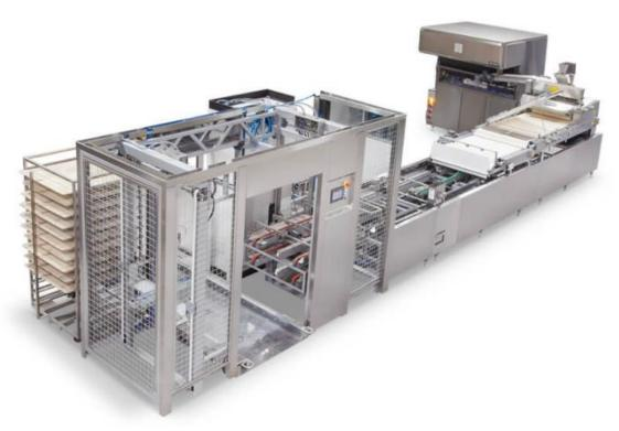
A major step up from our basic bread plant is the PROMAC fully automatic bread plant. The shaped dough coming from the Industrial Long Molder are spread out on to wooden pallets or trays in a single, double or triple row as demanded. Simultaneously unloading empty pallets or trays while loading the full pallets or trays on to the trolleys, full trolleys are then pushed out of the system and the empty new trolley is positioned in front of the loader.
