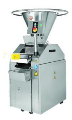
Main chassis is made of steel, dividing drum is made of chrome plated steel and the piston chamber is made of stainless steel. Anticorrosive piston, 24V control board, easy motion due to heavy duty casters, closed lubrication system. When machine is stopped it always stops at discharge point. Motor power transfer is done by pulley and belt system. Standard dough funnel has a capacity of 154 lbs. and the large funnel 308 lbs.
