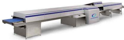
Speed is adjustable by converter. Pens are quipped with small rollers in stainless steel. Central zone of the tunnel is totally isolated to guarantee the maximum return of the refrigerating equipment. In the lower part are positioned the 2 evaporating batteries, while 2 fans with external rotor guarantee silence and elevated performances in terms of air flow. Fans are mounted on hinges to allow a better accessibility.
