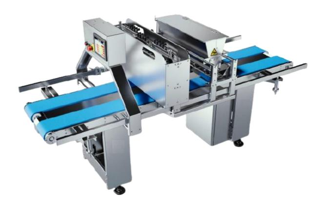
The Seed-O-Matic is a full automatic sprayer and seeder used in our bagel, roll, sandwich and hamburger line or as an independent stand-alone equipment. Machine is controlled by a HMI/PLC system with receipe saving.
