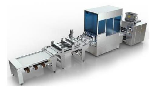
The PROMAC Hamburger and Sandwich Line consists of the Head Machine, Intermediate Proofer section, Dough Processing section and finally the Tray Loading section making it a complete line that can easily produce up to 7000 pcs/hour. Stamping section is optional.
